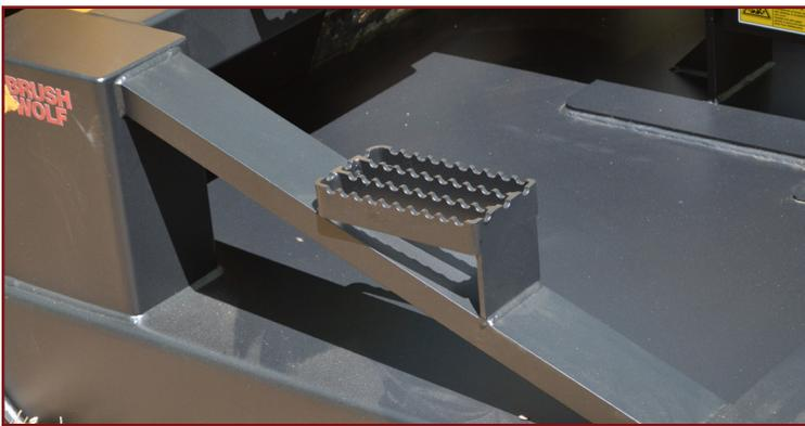
Step plate for easy entry into skid steer
